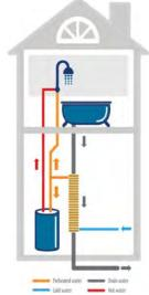
EcoInnovation's ThermoDrain™ drain water heat recovery units
